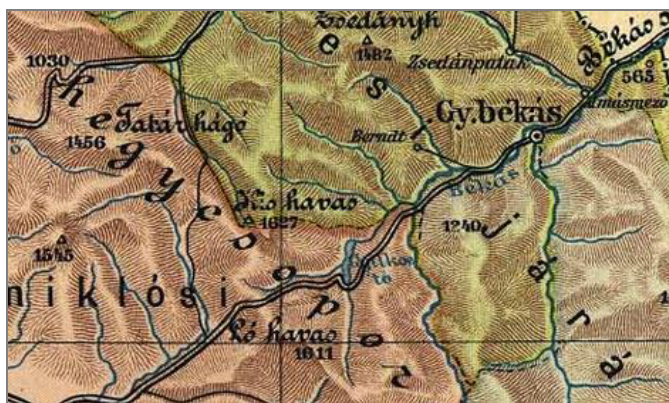
Fig. 1 Part of the test area with hachure lines
