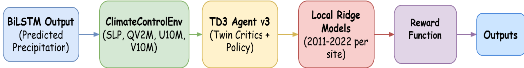
Fig. 4. Architecture of the TD3-based control framework coupled with BiLSTM-MLP forecasting.
