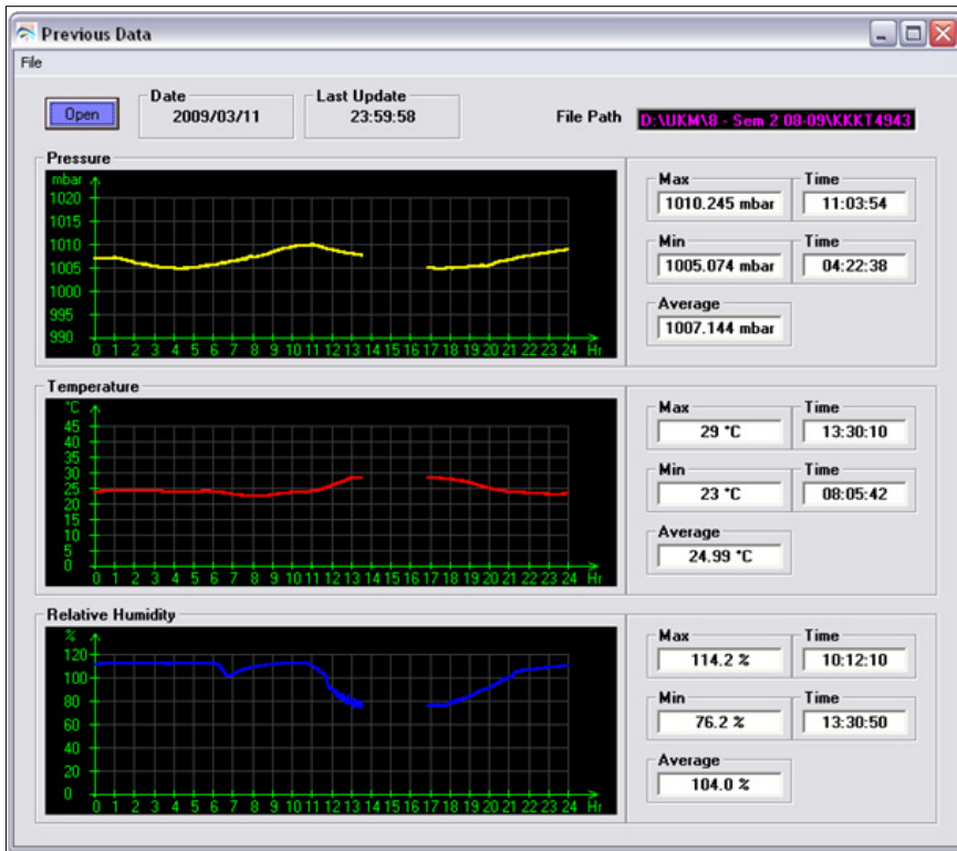
Fig. 6 Missing data due to the electricity problem has been handled by UAWS.
